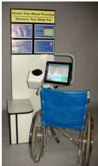
Figure 4 – The design allows unaided wheelchair accessibility. For photo clarity, no person is shown in the wheelchair.
