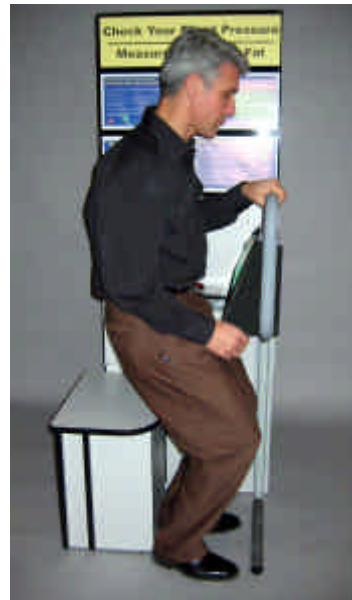
Figure 3 – The steel pipe provides a “grab bar” to assist the aged to stand up after a test.
